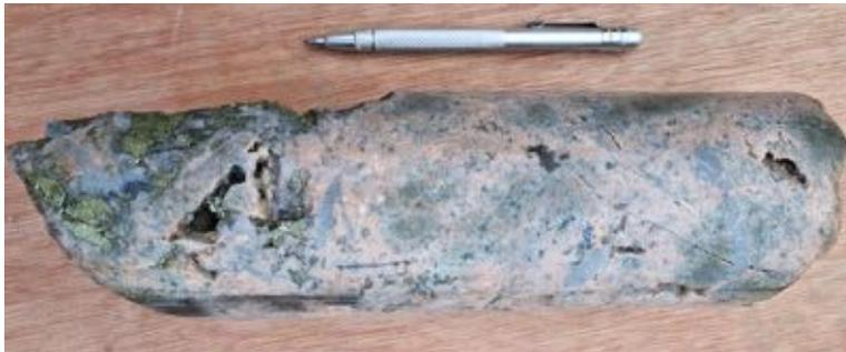
Figure 2 - 229m – Dacite porphyry breccia: intense potassic alteration (pink) mostly as halos around type A veinlets, quartz with chalcopyrite, molybdenite veinlets, disseminated molybdenite (grey speck) and chalcopyrite.
