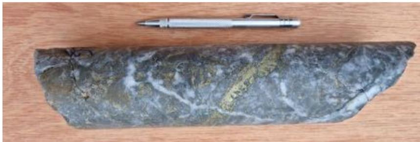
Figure 3 – 626m - Silicified dacite porphyry breccia: phyllic alteration with local potassic overprint. Several generations of quartz veining and chalcopyrite veining, with disseminated molybdenite and chalcopyrite.
