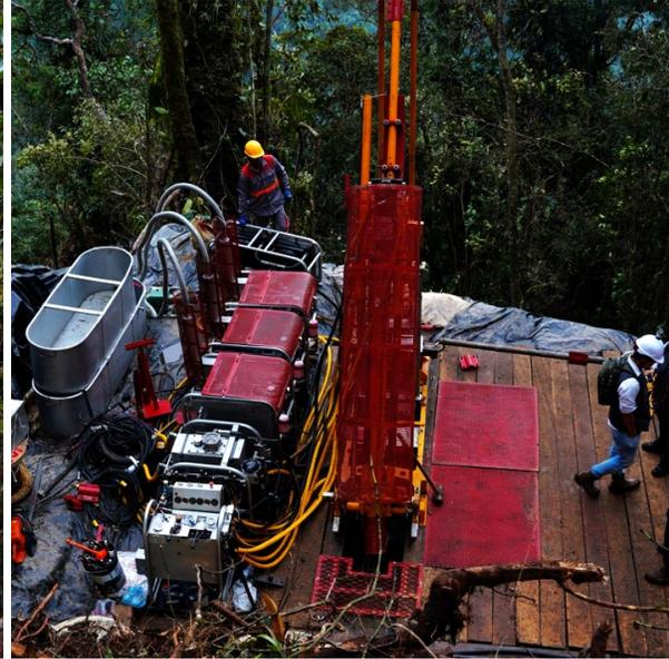
*Photo 2 – KD-1000 modular drill setup on first drill pad. Wood platform on earthen floor.*
