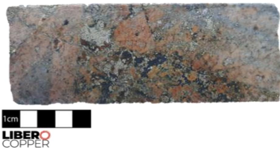
**Figure 1** – Magmatic-hydrothermal breccia with bornite, magnetite, quartz and K-spar matrix. Core from Mocoa, with potassic alteration and high magnetite content (222 metre depth).
