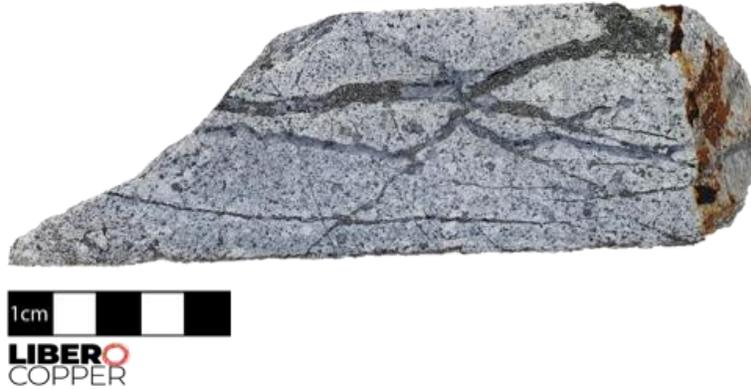
**Figure 4** - Transitional sericitic alteration are overprinting the prograde potassic alteration, where D-type pyrite-bornite-hypogene chalcocite veinlets associated with white sericitic alteration are overprinting and cutting the A-Type and B-type veinlets (132 metre depth).
