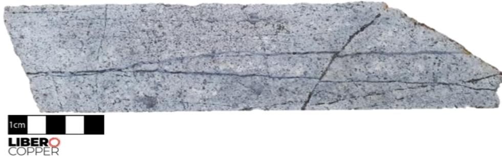
**Figure 2** - Transitional sericitic alteration overprinting prograde potassic alteration, low magnetite content (134 metre depth).
