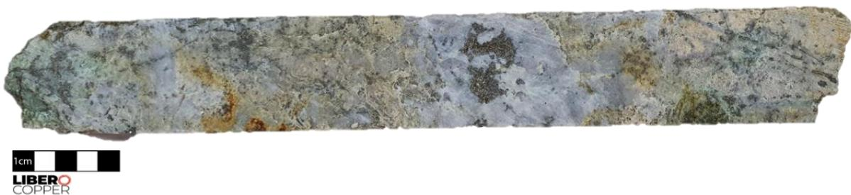
**Figure 6** - Magmatic-hydrothermal breccia with a muscovite-pyrite rich matrix (194 metre depth).
