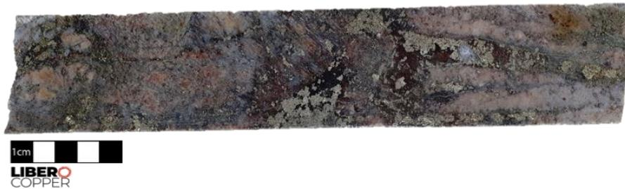
**Figure 5** - Magmatic-hydrothermal breccia with bornite, magnetite, quartz and K-spar matrix, with potassic alteration and high magnetite content (214 m depth).
