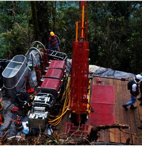
Photo 2 – KD-1000 modular drill setup on first drill pad. Wood platform on earthen floor.
