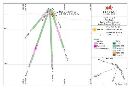
Figure 1: Cross-section of the 2020 RC drill holes at the Terry target  $\,$
