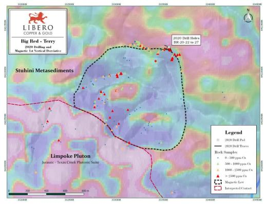
**Figure 2**: Locations of the 2020 Terry drill holes and surficial samples relative to the property scale airborne magnetics and the position of the Texas Creek Limpoke Pluton.
