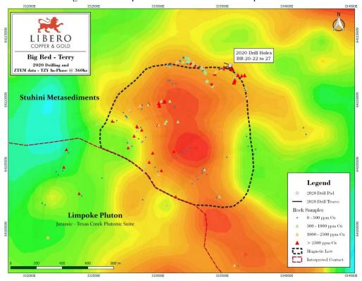
**Figure 3**: Locations of the 2020 Terry drill holes and surficial samples relative to the property scale electromagnetic (ZTEM) signatures, and the position of the Texas Creek Limpoke Pluton.
