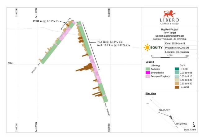
Figure 1: Cross-section of drill holes BR-20-23 and BR-20-27
