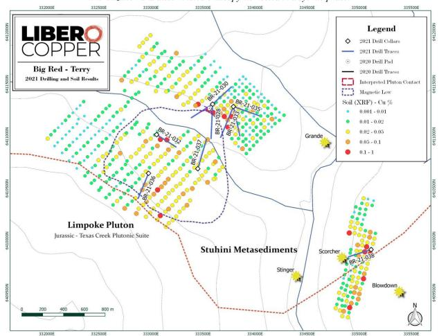
Figure 3: Plan map illustrating the distribution of drilling at the Terry target and the XRF Cu-in-soil results from the soil sampling programs.
