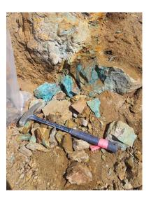
**Figure 2**: Photograph of mineralization observed in the new Scorcher showing strong malachite and chrysocolla mineralization and disseminated chalcopyrite hosted in a syenite phase.
