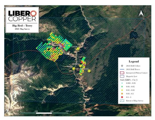
Figure 1: Plan map illustrating the coverage of the new magnetic survey, pXRF soil sample results and the 2021 drill program on and around the Terry Target.
